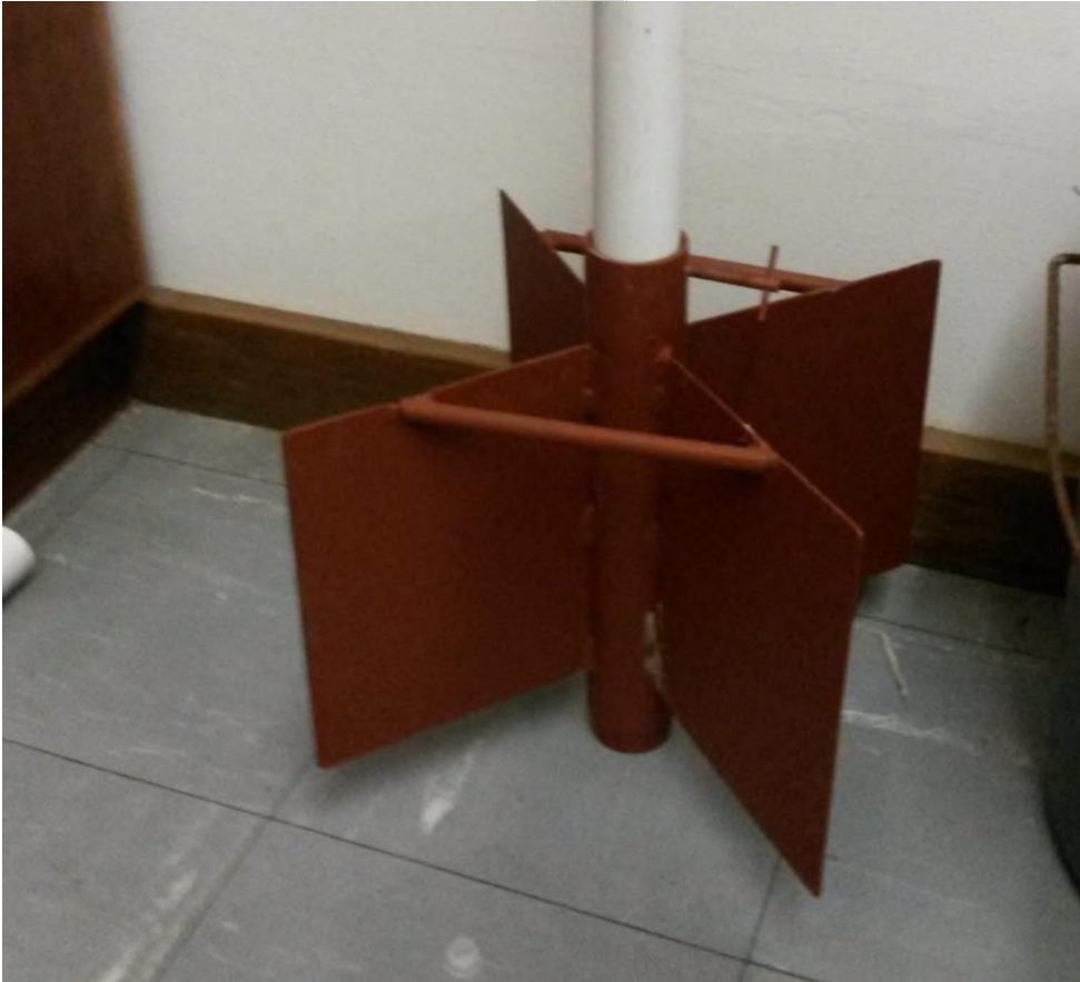
Figure 3.1: The 35.5 cm metal stand painted with Duram NS4 Anti Rust Coating Red Oxide along with the white PVC pole.
