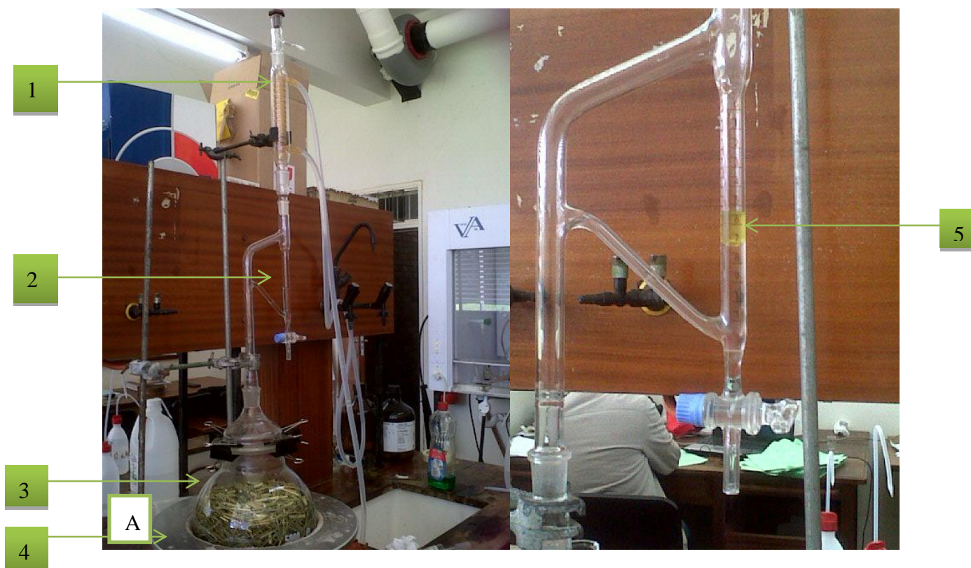
Figure 2-3: Clevenger apparatus set-up for hydrodistillation of C. validus
