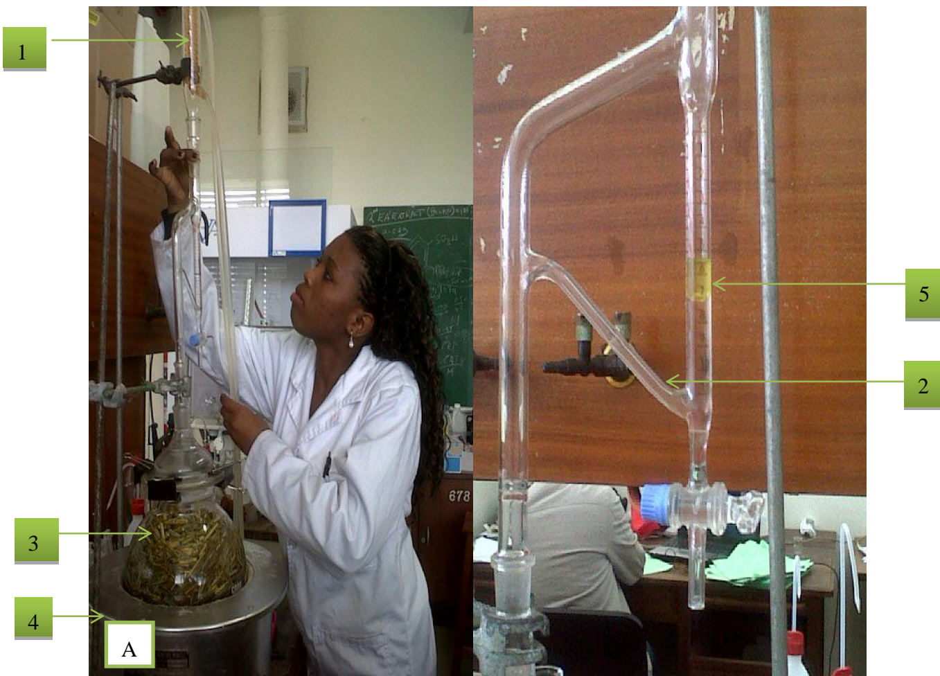
Figure 3-3: A: Clevenger apparatus for hydrodistillation of H. hirta
