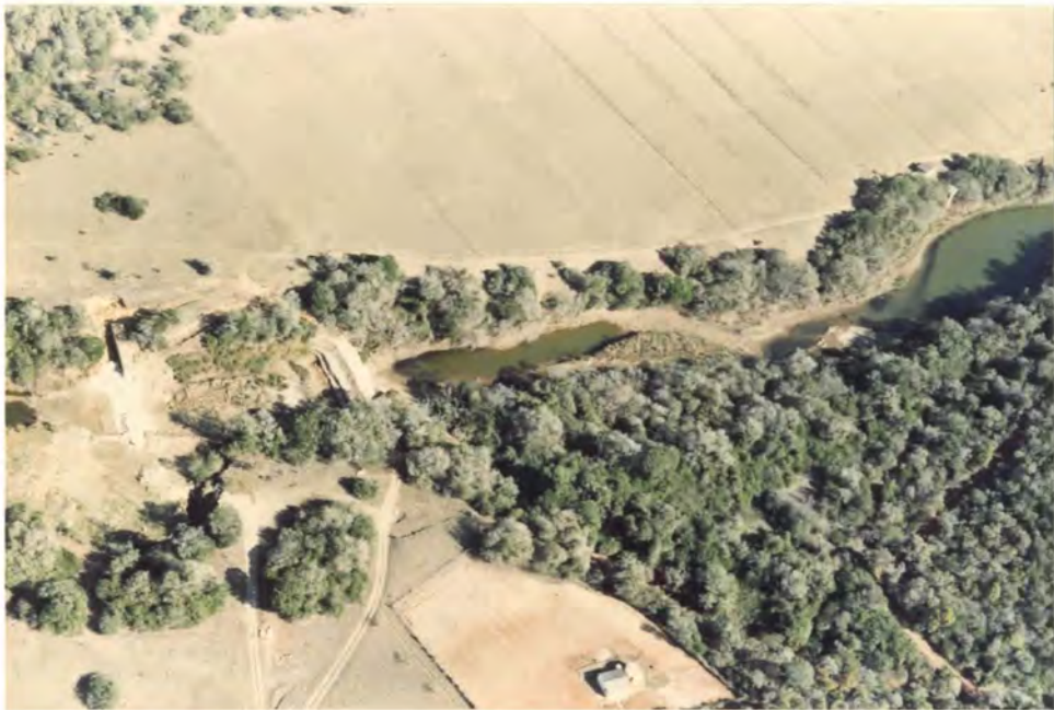
Figure 4. The "Ebb & Flow" of the Kowie River showing the old damaged and the new weir and Station 1 on upstream (RH) side of photo. Note low water level after 16 months of no flow.
