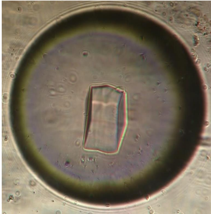
Figure 3.2: Faceted hexagonal ice crystal of Lepidonotothen squamifrons at the hysteresis freezing point.
