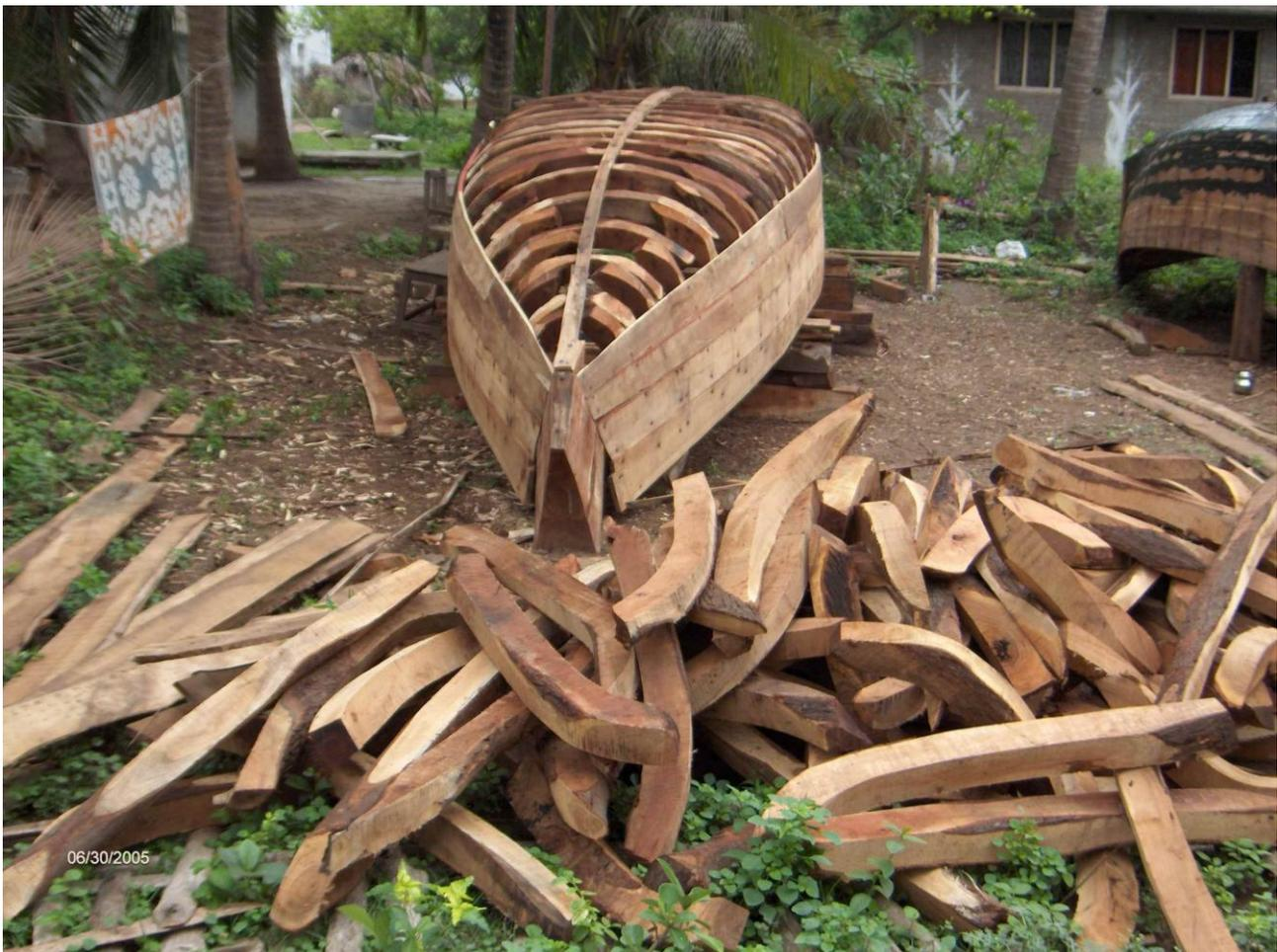
**Figure 18. Boat construction in Sitarampuram, using *Prosopis* wood.**
