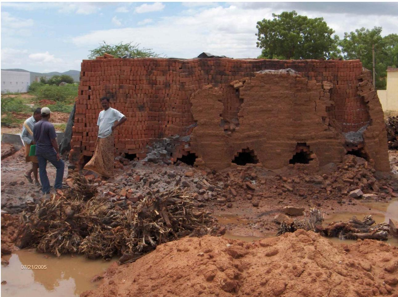
**Figure 17. Baked bricks with *Prosopis* roots used for the burning process.**
