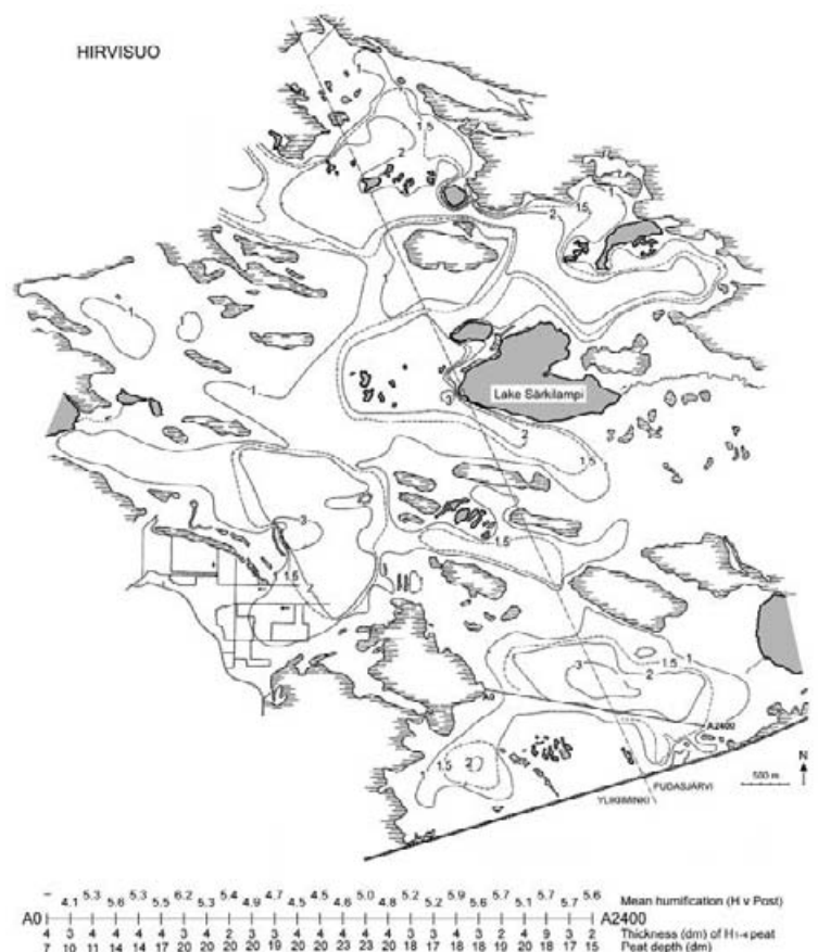
Fig. 1. Peat depth (metres) of Hirvisuo detected by ground radar. Transect (A0 – A2400 m) at the southern mire part exaggerated in the figure bottom. Mineral soil areas marked by horizontal line shading, lakes and mire pools by grey (Modified from Hänninen 1988).
