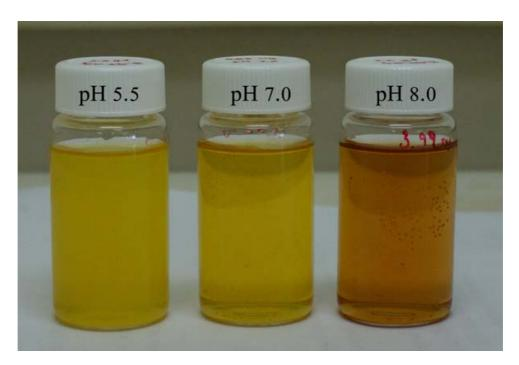
Figure 3-23 Extracts for stability under pH variation test at week 0
