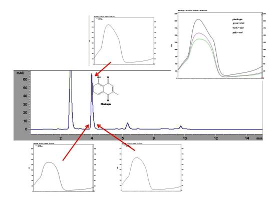
Figure 3-15 UV absorption spectra of plumbagin in P. indica root extract
