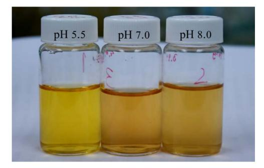
Figure 3-24 Extracts for stability under pH variation test after 16 weeks storage
