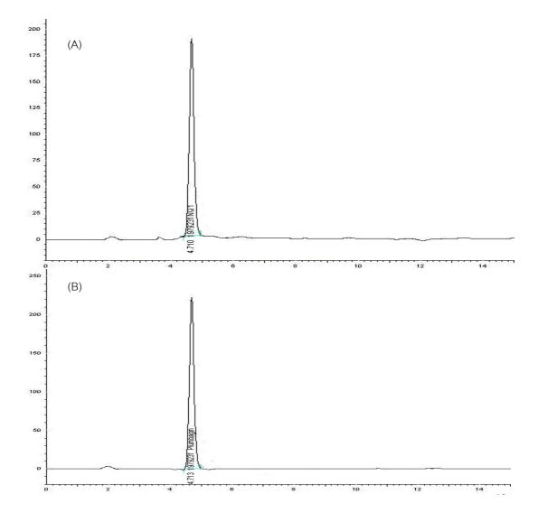
Figure 3-3 HPLC chromatogram of NQ 1 (A) compare to plumbagin (B) determined by the developed method; mobile phase consist of methanol and 5% aqueous acetic acid (80:20 v/v), flow rate 0.85 ml/min and detection wavelength set at 260 nm
