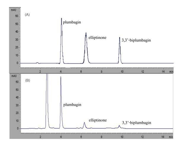
**Figure 3-14** HPLC-chromatograms of standard naphthoquinones (A) and naphthoquinone-rich *P*. *indica* root extract (B)
