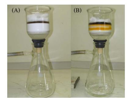
Figure 2-2 Vacuum silica gel chromatography (A) packed column before elution (B) after elution with a mixture of hexane and ethyl acetate
