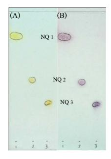
**Figure 3-2** TLC chromatogram of (1) NQ 1, (2) NQ 2 and (3) NQ 3 developed in hexane and ethyl acetate (9.6:0.4 v/v), (A) before spray with 10% KOH and (B) after spray with 10% KOH
