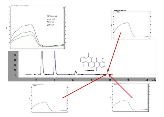
Figure 3-17 UV absorption spectra of 3,3'-biplumbagin in P. indica root extract
