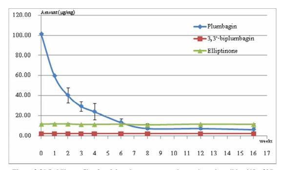
Figure 3-28 Stability profile of naphthoquinone content under accelerated condition ( $45 \pm 2^{\circ}$ C and 75% humidity)
