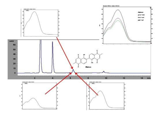
Figure 3-16 UV absorption spectra of elliptinone in *P. indica* root extract
