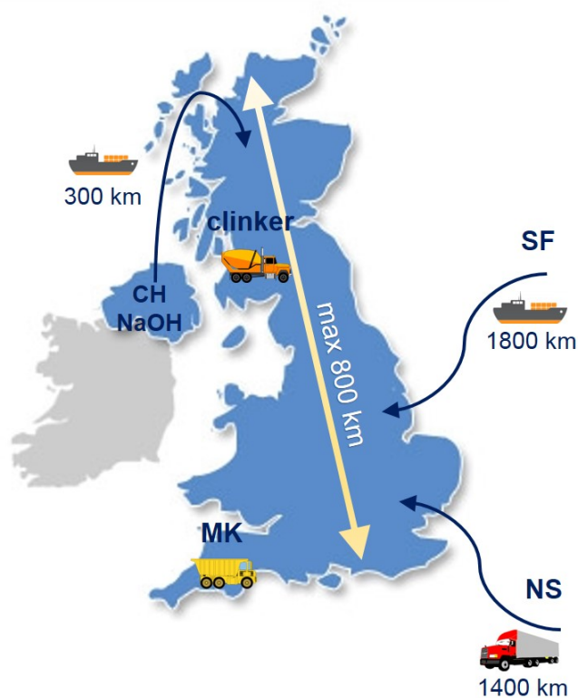
Figure 2: Diagram of transportation mode and average distance for raw materials in and to UK. Silica fume (SF) is supplied from Norway, nano-silica (NS) from Germany, calcium hydroxide (CH) and sodium hydroxide (NaOH) from Northern Ireland (UK), metakaolin (MK) and Portland clinker are available in mainland UK.
