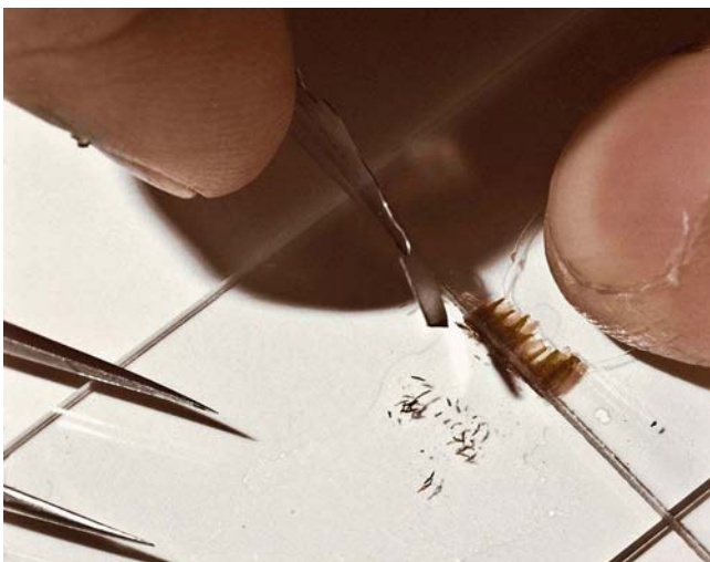
Figure 110. Cut sections along edge of top slide in double slide sectioning technique of Sean Edwards. Note the alignment of multiple stem pieces under top slide. Photo by Sean Edwards.
