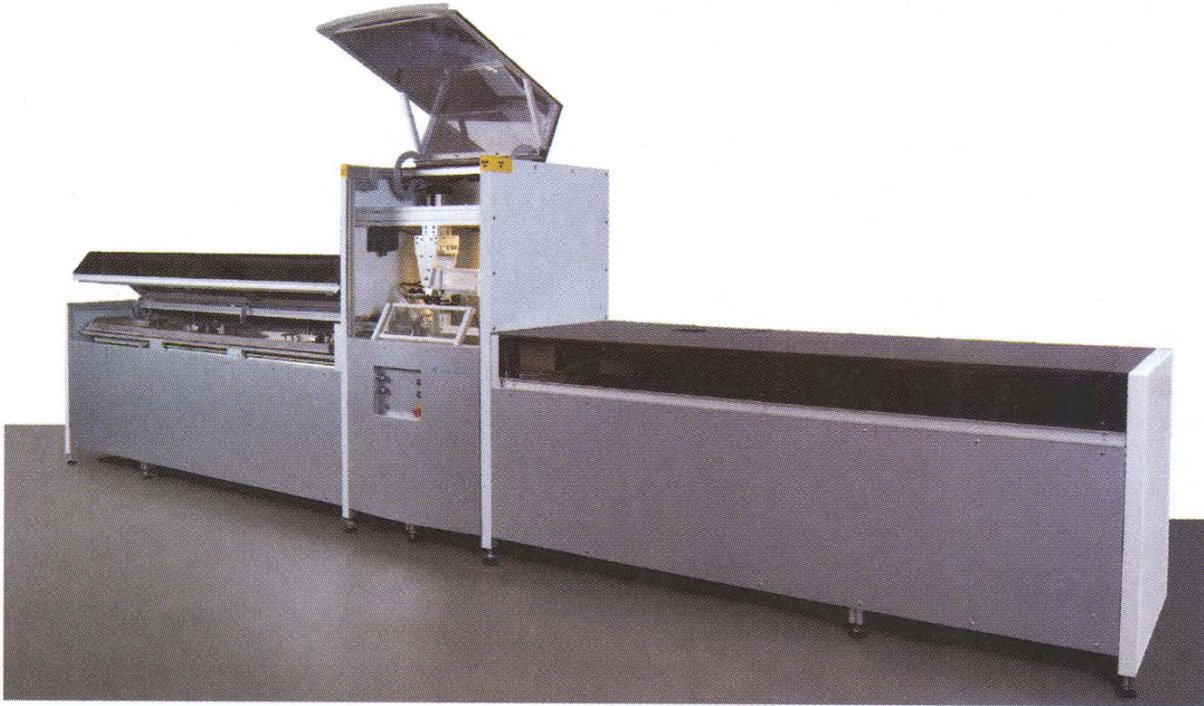
Figure 3.18: ITRAX core scanner (Figure 1; Croudace et al., 2006).
