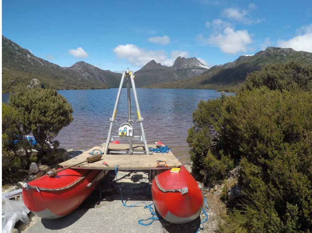
Figure 3.5: University of Melbourne Palaeoecology Laboratory coring platform equipped with two pontoons, a wood deck and the Nesje tripod (by: Kristen Beck, 2015).
