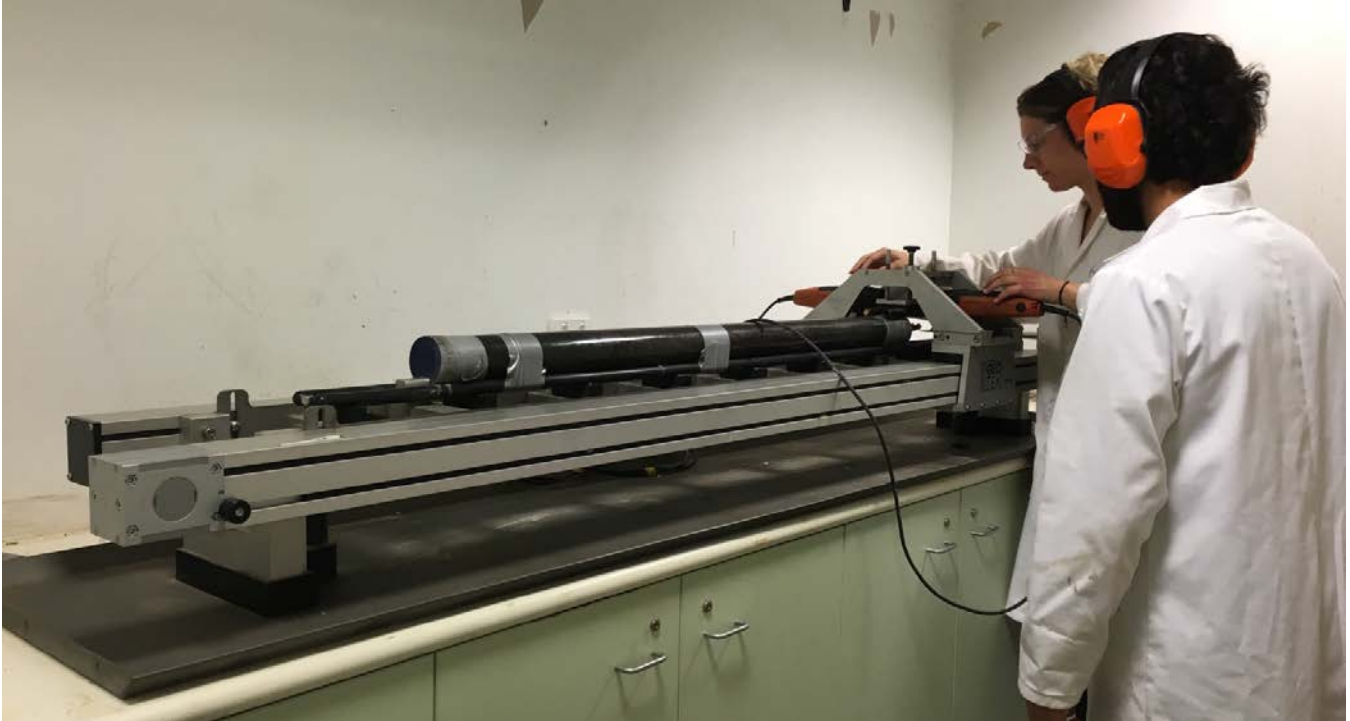
Figure 3.11: Core splitter at University of Melbourne. Splitting a Universal Core from Rebecca's Lagoon, northwest Tasmania (by: Bianca Dickson, 2016).
