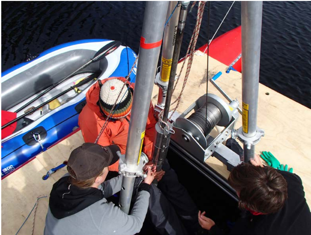
Figure 3.7: Attaching the aluminium chamber to the Nesje coring head at Paddy's Lake (by: Alexa Benson, 2014).
