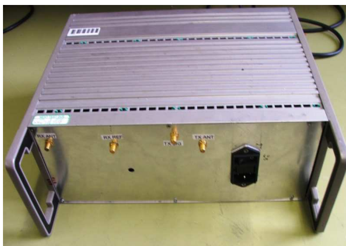
Figure 5.2 Portable rack with RF components
