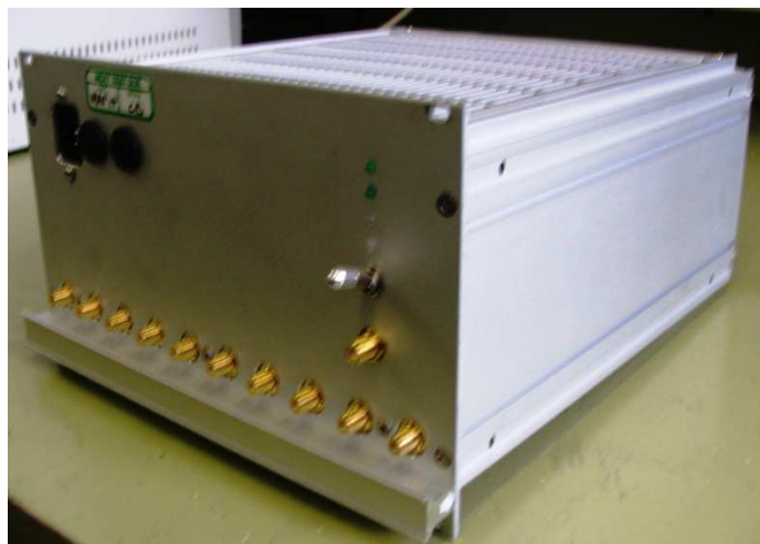
Figure 5.14 Rubidium clock generation and distribution block
