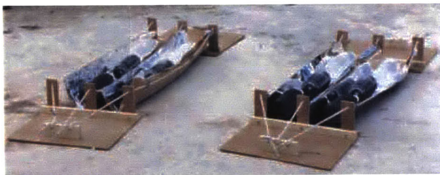
Figure 3.2 Solar reflectors, Left: aluminum foil, Right: aluminum mylar
