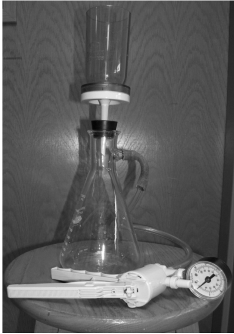
Figure 19: Filter apparatus used to process samples. One-liter samples were passed through 3 \mu m filters. The hand-pump provided gentle filtration catering to possible trophic forms of amoebae or resistant cyst forms.
