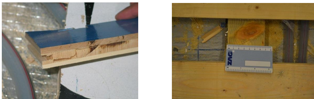
Figure 9. Left: Not properly supported wear layer. Right: Size of knots and slope of grain.
