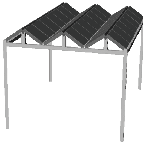
Figure 2. Platform that was placed at the study site containing 42 tiles, sponges were attached on every tile. Size platform: 2,5m x 1,6m x 1,2m.
