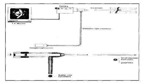
Figure 3-3 Simple way of recording the root growth in the perforations on photo or movie camera. The light that has passed the glass fibre light connector is "cold"(from Smits, 1994)
