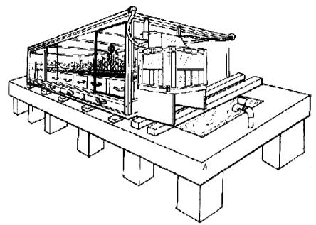
Figure 2-3 In "controlled" conditions the water was circulated through an automatic system to keep inside air temperature between  $27^{\circ}$  and  $30^{\circ}$  C. A = concrete table, B = small aquarium pump, C = thermostat.
