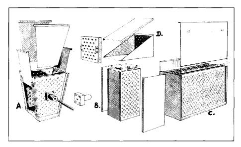
Figure 3-1 Four types of "performs" suitable for use with the horizontally perforated soil system (from Smits, 1994)
