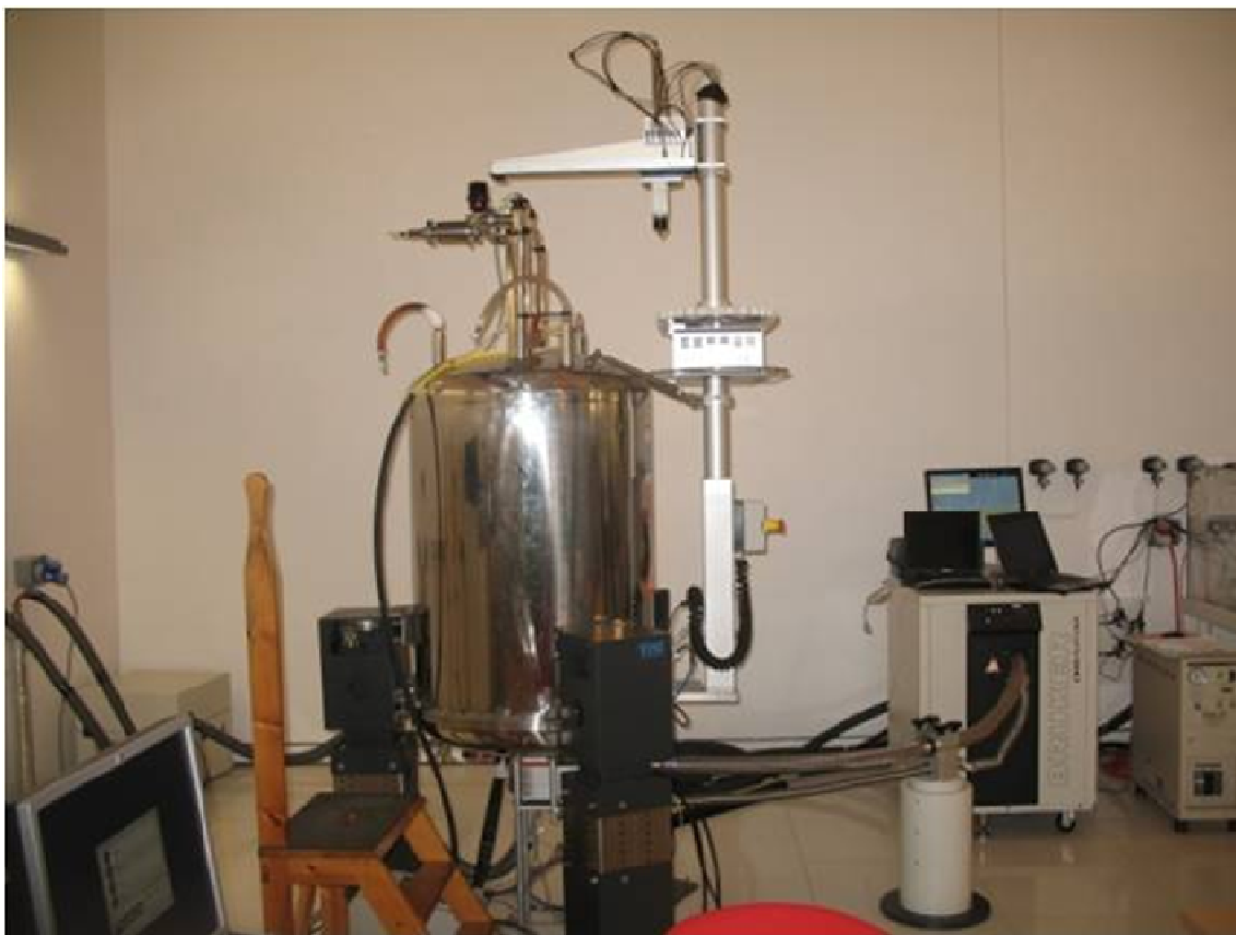
Figure 5.1 Bruker DRX-500 MHz NMR spectrophotometer used to obtain ^1\text{H} NMR spectra. Image courtesy of J. Byrne, NERC metabolomics facility, University of Birmingham.
