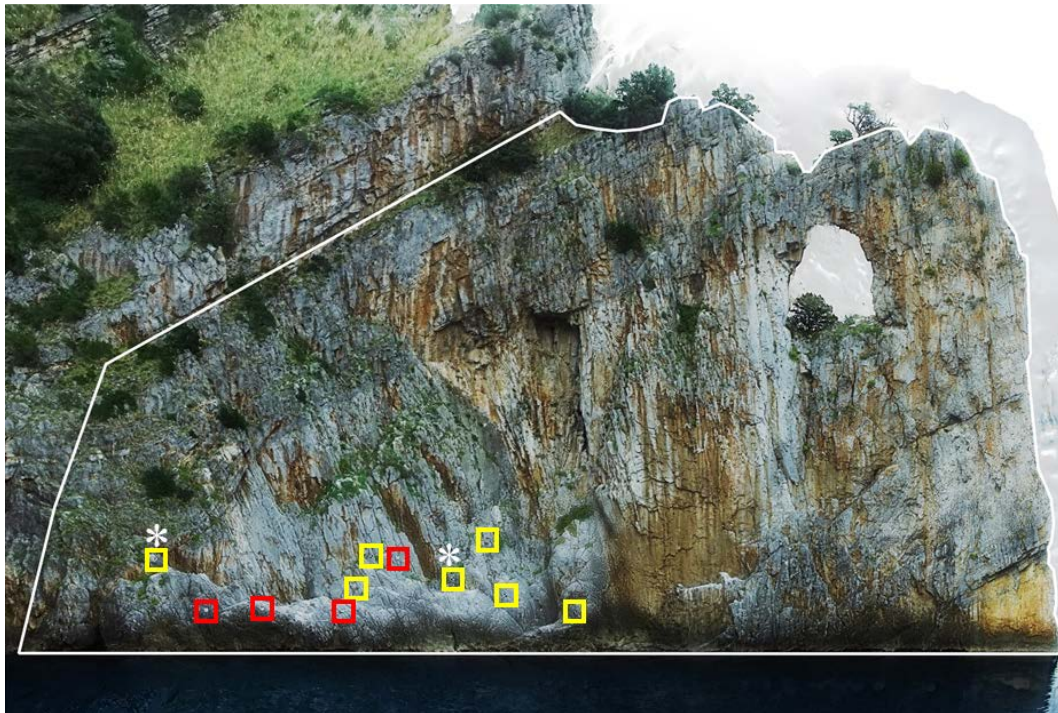
Figure 1. Orthomosaic of the analysed cliff. The Total Surface (TS) of the cliff is delimited by a white line. At the bottom of the cliff, the seven Ground Control Point (GCP) targets and the four USAF (United States Air Force)-1951 Resolving Power targets are highlighted by yellow and red squares respectively. The two asterisks indicate the GCPs used for checking image scaling.
