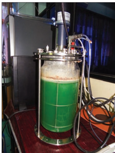
Mass production of Ps04 using biofermenter: the cells were heat killed and spray dried. The spray dried form was estimated for activity and packed
