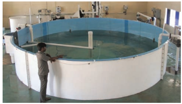
Imported RAS facility showing the main reservoir for broodstock holding
