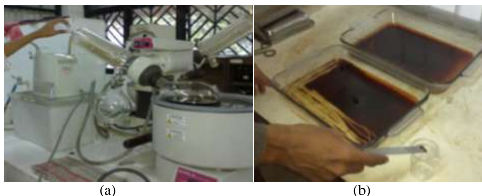
Figure 3. Paste produced process (a) Liquid extract was condensed by using rotary evaporator (b) gel-like extracts called paste
