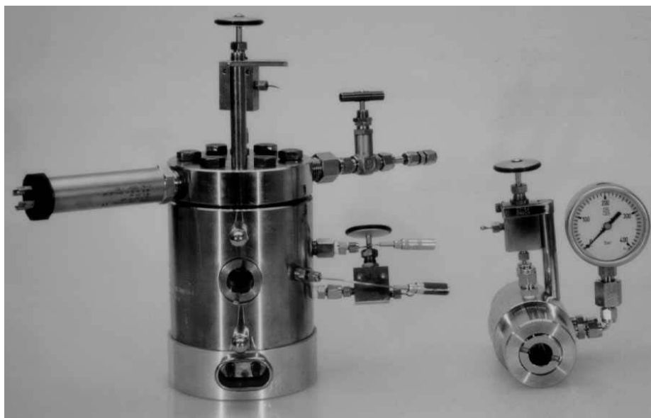
Figure 2-5: High pressure reactors used for exploratory studies on chemical synthesis using scCO 2 .
