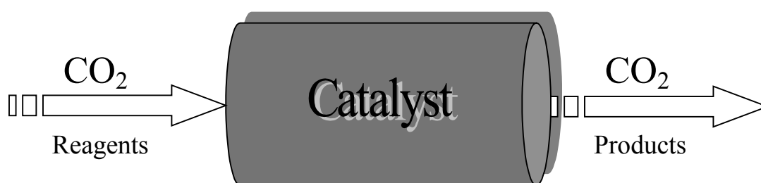
Figure 1-4: Ideal catalyst cartridge for multipurpose catalysis in a generic multiphase catalytic reaction.
