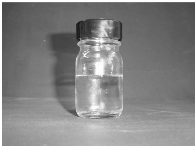
Figure 2-10: Colorless sample of the ionic liquid [BMIM][PF 6 ].
