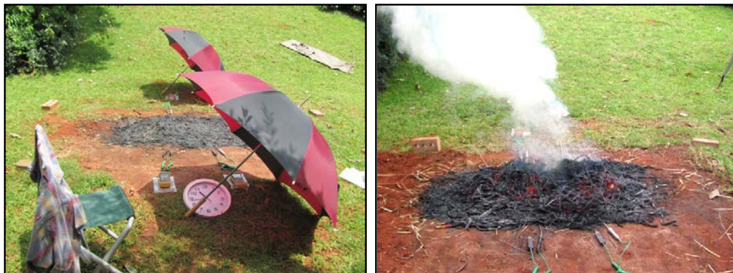
Figure 8.1 Burning of sedge bedding, experiment set-up and fire (Series 1 Bed 1).
