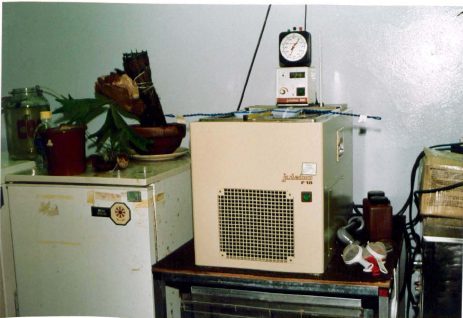
Figure 2.6 A thermostatically controlled 50 litre water bath for heat or cold shock treatment.
