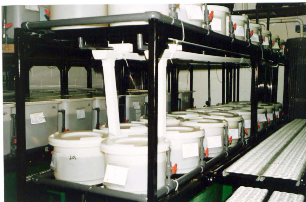
Figure 2.3 Fry and fingerling rearing system.
