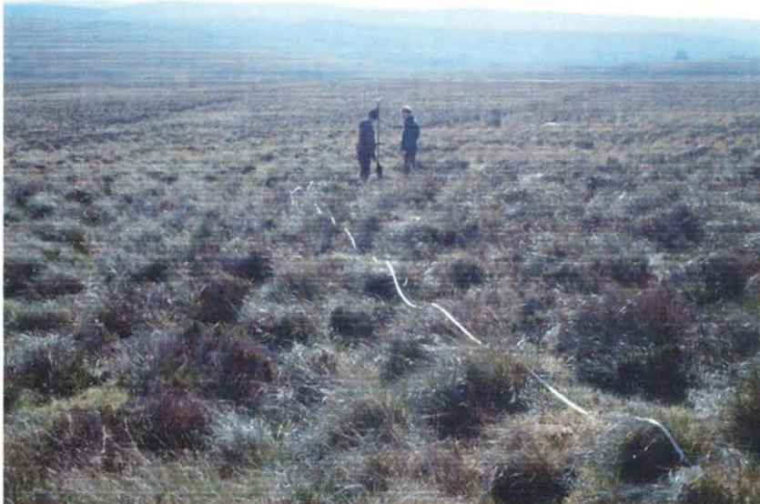
Figure 4.4: Peat samples were taken using a Russian corer to obtain a detailed record of peat stratigraphy
