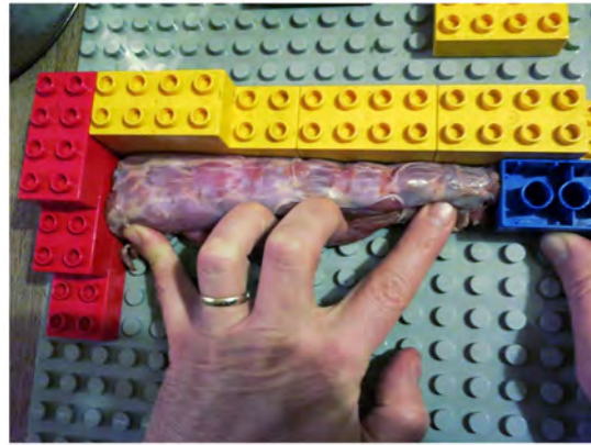
Figure 7. Measurement rig for necks. Measurement rig for intact turkey necks, constructed from Duplo bricks and baseboard. The neck is pushed into the angle between the back wall (yellow) and the left wall (red), and held straight along the back wall. The marker brick (blue) abuts the end of the neck: the distance between the left wall and the marker brick is the length of the neck between perpendiculars. doi:10.1371/journal.pone.0078214.g007
