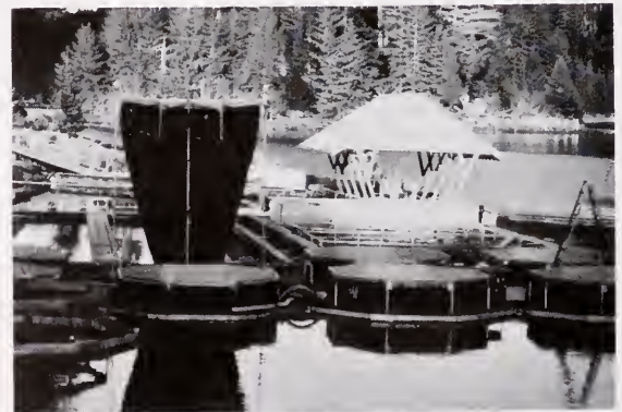
Figure 6. Vertical raceway hoisted from its flotation collar (left center). (Photo courtesy of NMFS, LPW, Alaska).
