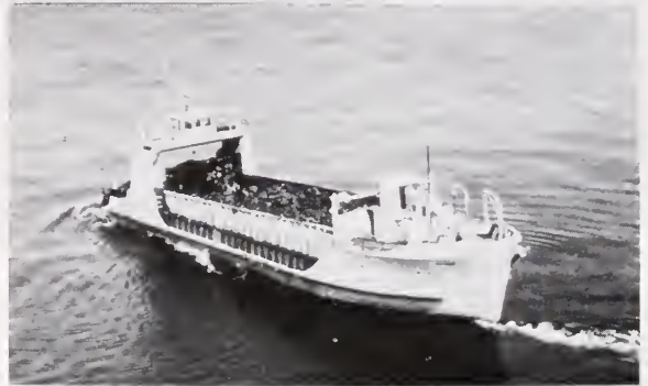
The modern harvester, Kelmar, loading giant kelp. The vessel is being pushed through the kelp forest by a bow propeller. (Courtesy of Kelco)
