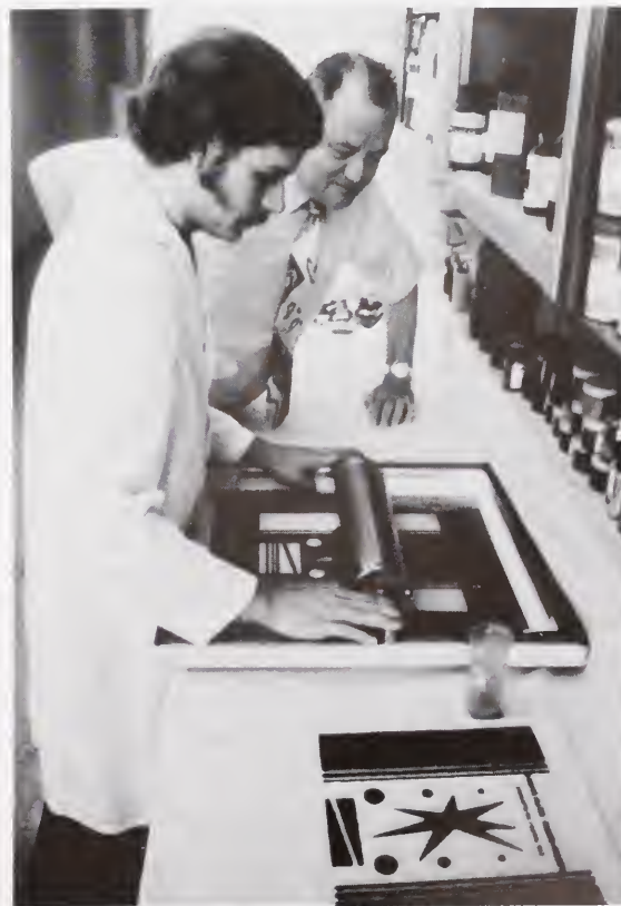
Textile print pastes containing algin provide excellent ink-migration control for fine line printing. (Courtesy of Kelco)
