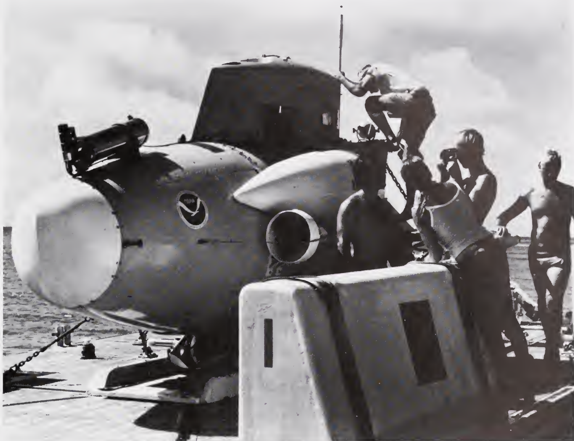
Conductivity and depth profiler (CDT) mounted (top, front) on Anderson Research Laboratory's submarine, Makali'i. Data are recorded on audio tape inside the vehicle for subsequent analysis.
