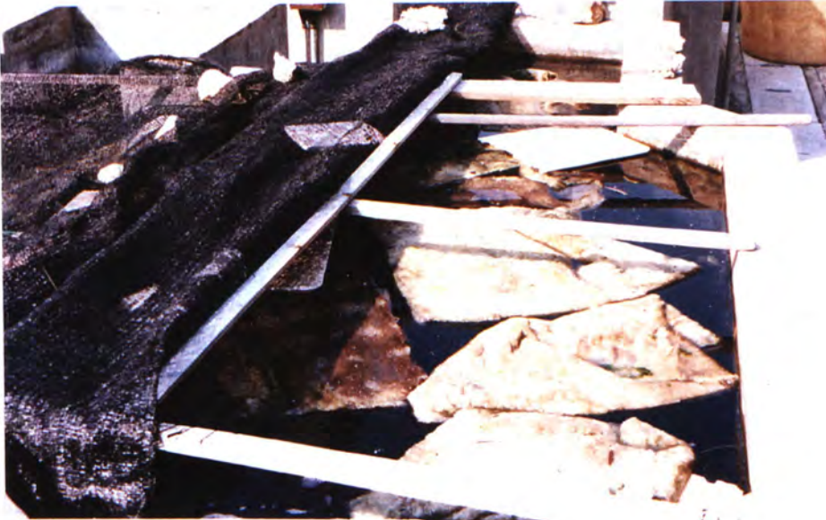
Figure 2.1 The outdoor concrete tanks in Marine Science Laboratory, The Chinese University of Hong Kong. A, the tanks are covered with sheets of perforated nylon net; B, pieces of fiber-cotton filter provide food and substratum for amphipods.
