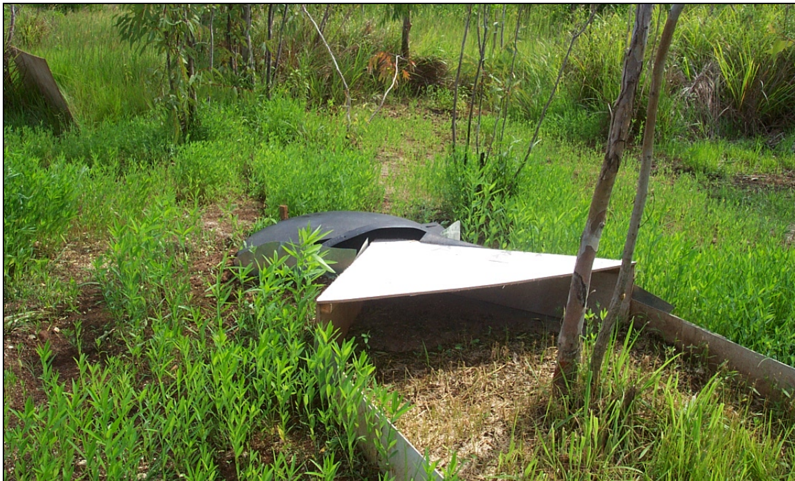
Figure 5-1. Runoff storage tanks at the downslope end of the erosion flumes.
