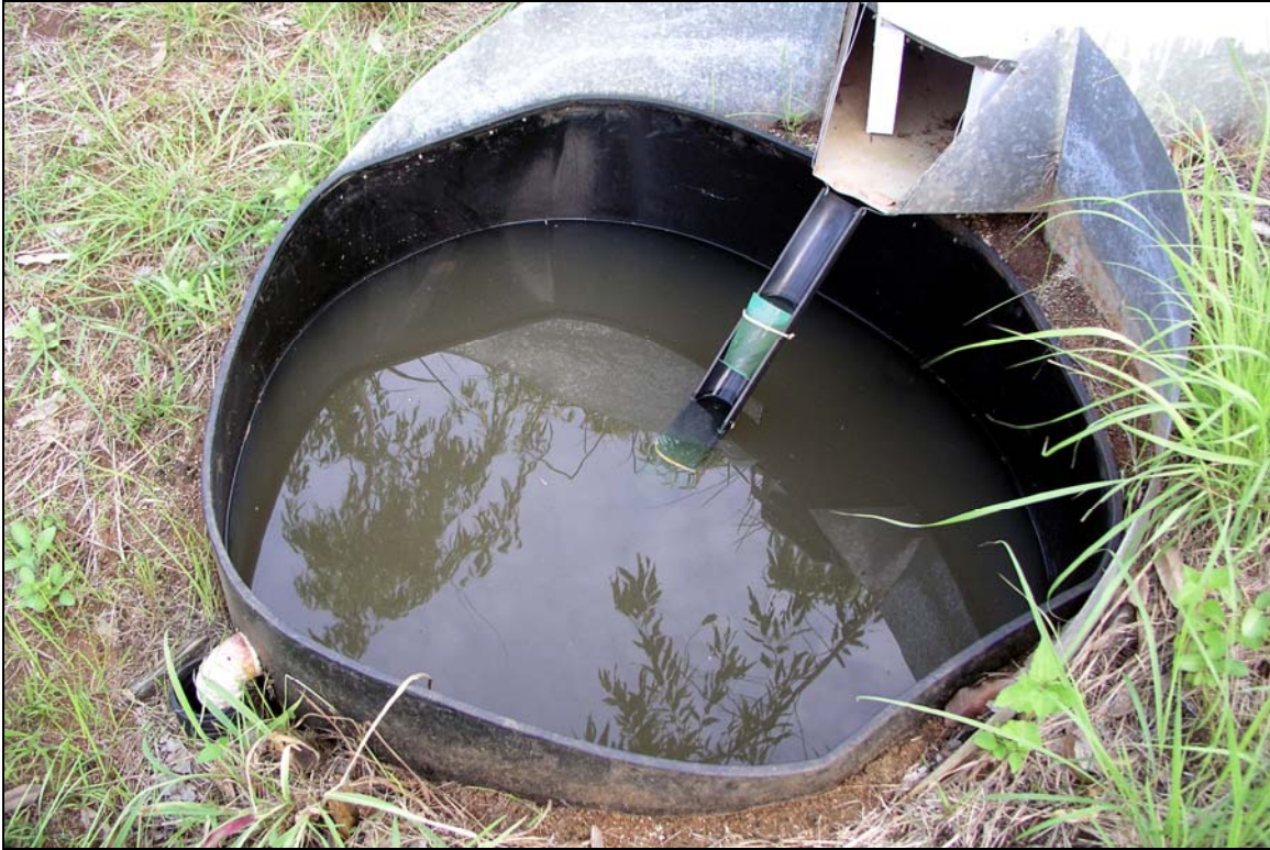
Figure 5-2. Sediment sampling apparatus in one of the runoff storage tank.
