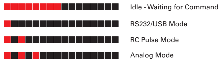
FIGURE 16. Normal Operation Flashing Patterns
