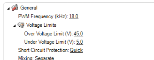
FIGURE 82. General Power Stage configuration parameters
