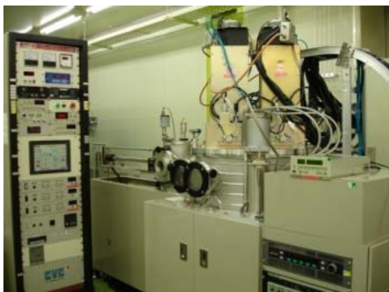
Fig. 3-5 DC magnetron sputtering machine for the deposition of NbTiN films in NiCT and typical deposition condition.
