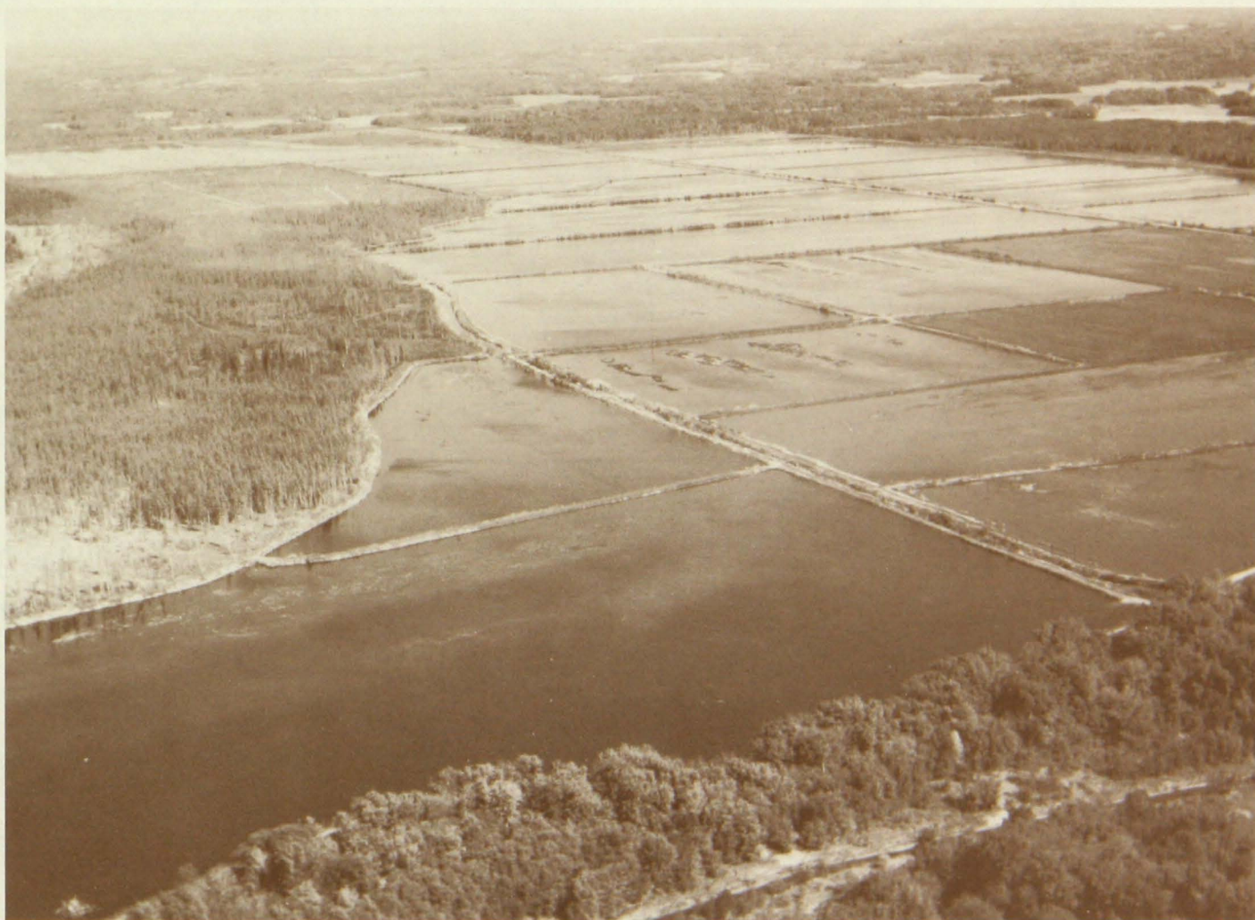
Figure 9. A layout of wild rice fields with water supply ditches in the upper right and center. The river from which the water is pumped is in the lower corner. The area covers about 700 acres.
