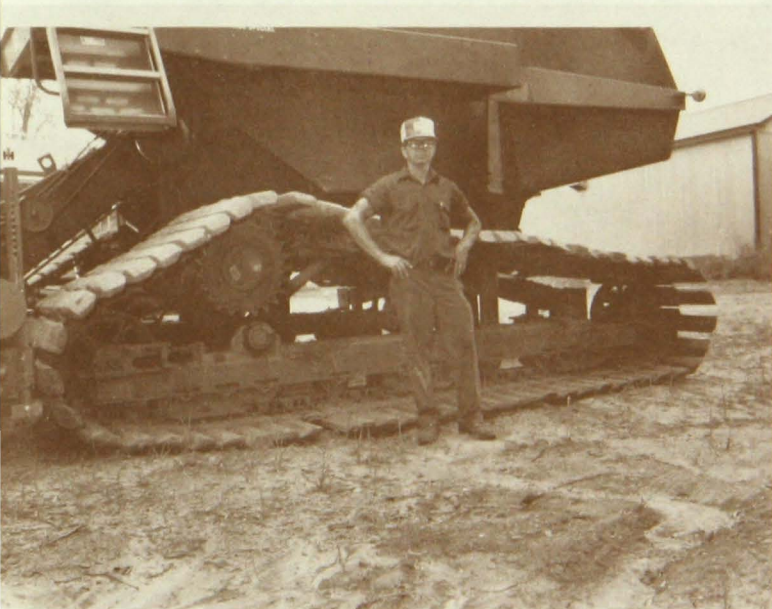
Figure 24. Combine with a full track system for wild rice harvesting.
