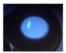
Figure 2.2: Adjusted X-ray beam shown on fluorescent powder.
