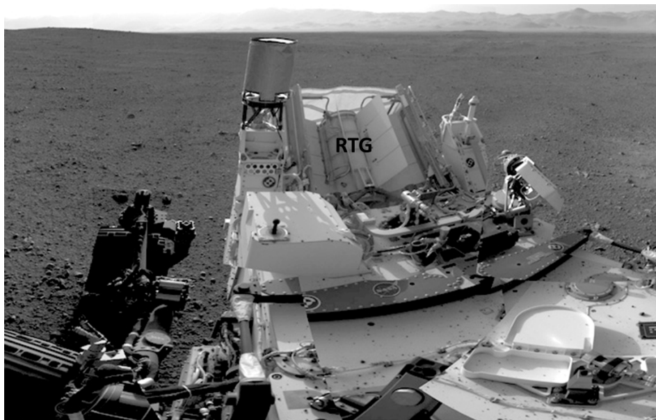
Figure 1.1: Self-portrait of the Mars rover Curiosity . The finned barrel shown with the label ‘RTG’ is the Radioisotope thermoelectric generator on board the rover that runs on improved thermoelectric materials based on PbTe/TAGS.
