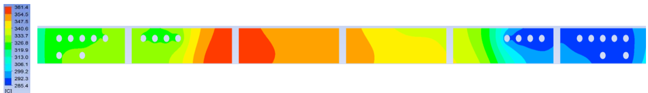
Fig. 52 – PbLi outlet temperature in a poloidal – toroidal plane (Sim IV)
