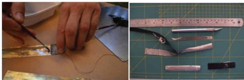
Figure 4 Dielectric electroactive polymer (DEAP) thoracic sensors project developed by A.Toomey, N.O'Connor and P. Stevenson-Keating in 2012. The industry standard sensors were taken apart and fabricated in-house to enable bespoke specification and integration into the sensing vest.
