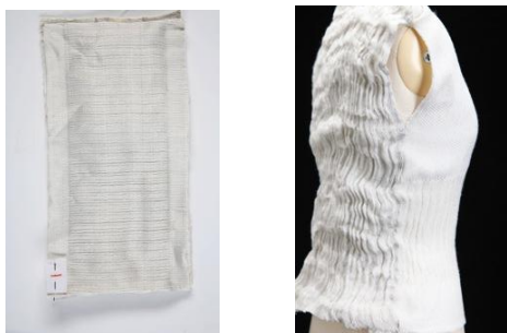
Figure 3 ‘Loom to hanger’ project developed by V.Kapsali and J. Stephenson at Middlesex University in 2008. The shrinking effects of wool in hot water were studied in combination with effects of weave and yarn structure. A 2D layered textile was engineered (left) that when exposed to hot water, transformed into a fully fashioned vest with design details without the need for further processing i.e. cutting and sewing (source V.Kapsali).
