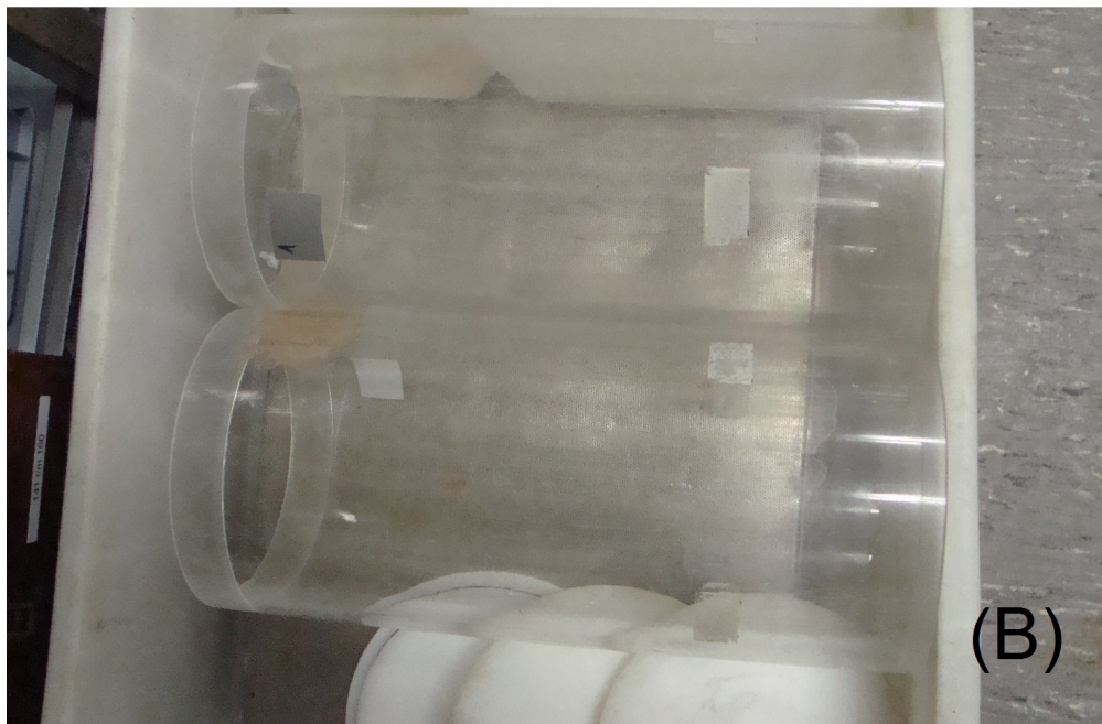
FIGURE H.4: A) A lid with different holes used to introduce the stirrer, sensors for digital records or pipettes for the Winkler titration; B) The perspex chambers ( d = 30 cm). All material provided by the Ecosystem studies department of the NIOZ-Yerseke.
