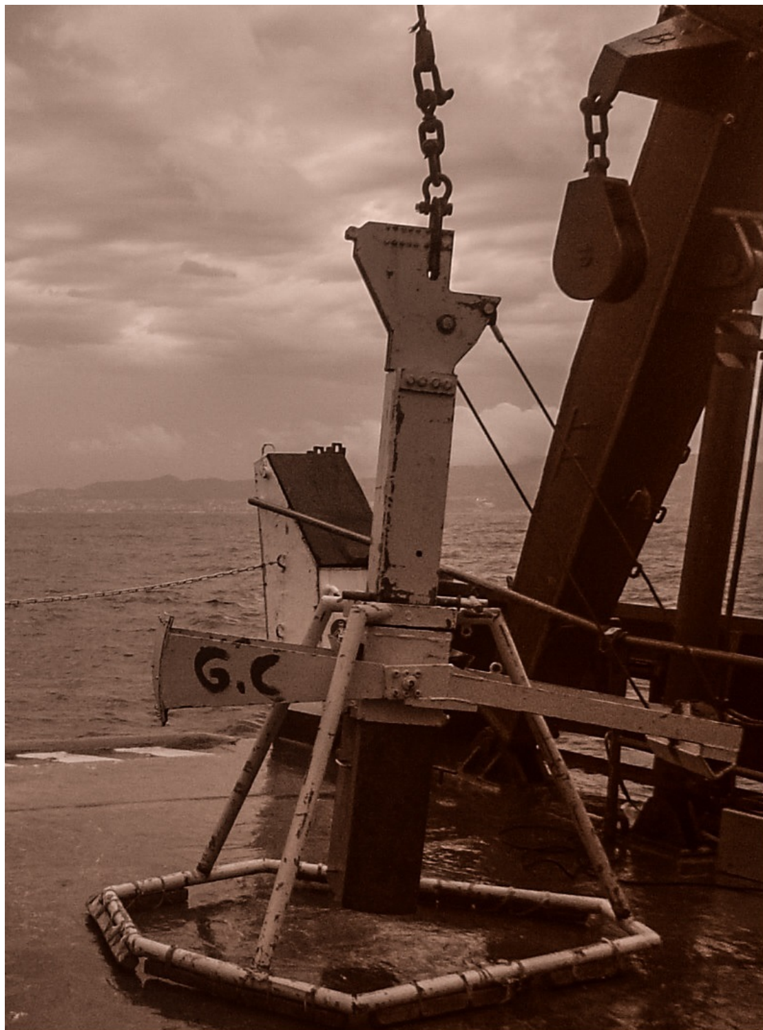
FIGURE H.1: Boxcorer. B/O García del Cid, Catalan Sea, BIOMARE October, 2007.
