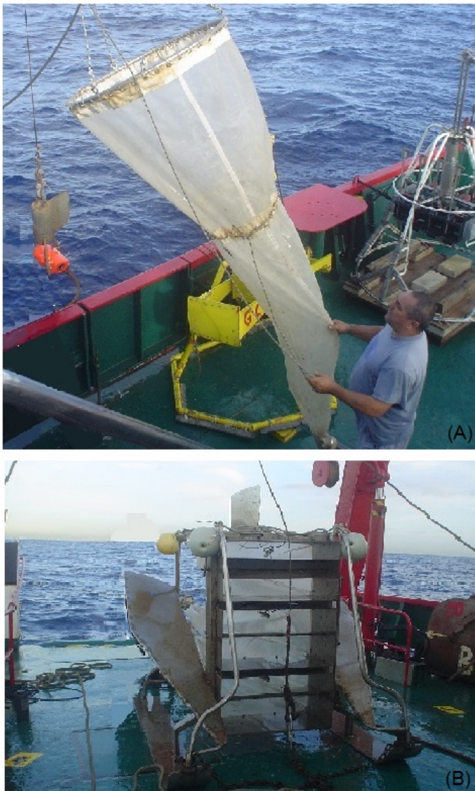
FIGURE H.3: (A) WP2 used to sample zooplankton and micronekton. (B) Suprabenthic sledge used to sample suprabenthos. B/O García del Cid, Catalan Sea, BIOMARE October, 2007.
