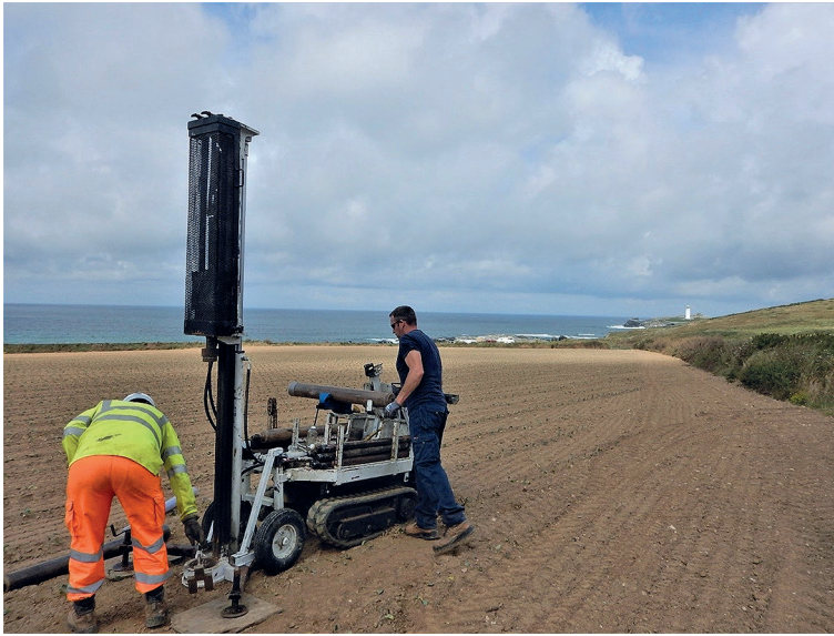
Fig 6 The percussion coring rig at T1/1 (Photograph: © M J Allen 2019).
