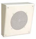
The MB8TSQ and MB8TSL speakers feature an all-steel surface-mounted enclosure with an 8 in. cone loudspeaker and multi-tap 4-watt 70V/25V transformer. The MB8TSQ is suitable for ceiling or wall mounting. The MB8TSL is designed primarily for wall mounting and its face is angled downward by 12.5 degrees.
