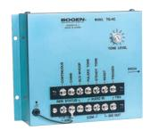
The TG-4C is designed to produce four different types of tones for use as alarm or announcement signals in paging systems. An audio signal can be routed through the TG-4C to allow easy installation in paging systems. During generation of the tones, the routed audio will be suppressed.
