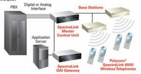
The SpectraLink 6000 System is a dedicated wireless voice system, providing the highest level of reliability and security with minimal administration and maintenance. The SpectraLink 6000 System is the preferred choice of more enterprises in the U.S. than any other wireless system available.
