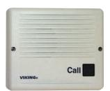
The E-10A and E-20B can be connected directly to a C.O. line or analog PABX/KSU station when used in conjunction with a hot-line dialer or programmed ring down circuit. When the "Call" button is pressed, the E-10A or E-20B will come off-hook and will remain off-hook until a CPC is detected or the pre-selected timeout has elapsed, the unit will then automatically disconnect. For outdoor or harsh environments, the E-10A and E-20B are available with Enhanced Weather Protection (EWP).
