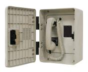
GAI-Tronics' industrial telephones are designed for those applications where standard telephones are not environmentally suitable. The auto-dial telephones are programmed to automatically dial when the handset is taken off hook. The phones have a detachable programming keypad, preventing unauthorized tampering of the pre-programmed phone number.
