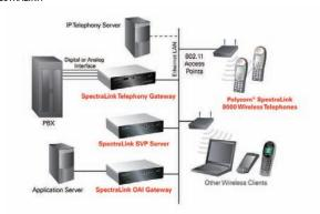
The SpectraLink 8000 System offers mobile voice over a converged voice and data network, which reduces costs and simplifies management while significantly improving employee mobility, responsiveness and productivity. The SpectraLink 8000 System provides the richest functionality while integrating with the broadest range of enterprise applications and networks.
