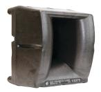
GAI-Tronics' Addressable Amplified Speakers are suitable for any permanent or temporary public address paging application. With its built-in amplifier circuit, rated 8 watts at 12 V DC, there is no need for a separate power amplifier, increasing system reliability by removing the single point of failure and creating a distributed amplified system. The addressable amplified speaker performs a self adjustment of its output volume based on the surrounding ambient noise level.
