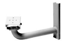
The EM1109/EM2000/EM2200 are medium-duty enclosure mounts designed for applications where mounting on a parapet or pole is necessary. These mounts can be used with Pelco enclosures having a 2-inch mounting hole pattern and are capable of supporting up to 40 lb. All three mounts feature a manually adjustable swivel head and a cable feed-through hole to conceal wiring. Multiple mounting holes on the tilt table provide 360 degree horizontal positioning of the enclosure.
