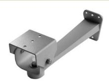
The EM1450 is a light-duty wall mount designed specifically for use with Pelco's EH3500 Series enclosures. Manufactured from die-cast aluminum, the EM1450 is capable of supporting a maximum load of 20 lb. (9 kg) and can be safely mounted to any vertical load-bearing surface.
