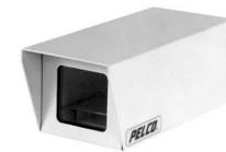
The EH100 Series are low-cost, light-duty, indoor camera enclosures designed for use with various cameras on the market. These enclosures will accommodate fixed focal length lenses or motorized zoom lenses. All aluminum construction and rugged powder-coated surfaces make the EH100 Series a lightweight, attractive camera enclosure for most indoor applications.
