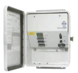
These power supplies provide 24 V AC output for one to four cameras. To compensate for voltage losses over long wire runs, 28 V AC outputs also are available on the WCS4-20. The power supplies have a selectable input of 120 or 230 V AC.
