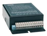
The KTD-83 is a data signal distributor that is designed for use in a Digiplex system. It is used when an RS-422 control signal must be dispersed along separate lines of 2 conductor UTP cable.
