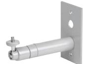
The C10-UM is a universal camera mount kit that includes all the components for wall, ceiling, or T-rail clip installations for most box type cameras with 1/4 x 20-inch mounting holes. The kit supports cameras weighing up to 7 lb (3.18 kg). The ball socket of the kit allows for 360-degree pan adjustment and 90-degree tilt adjustment.
