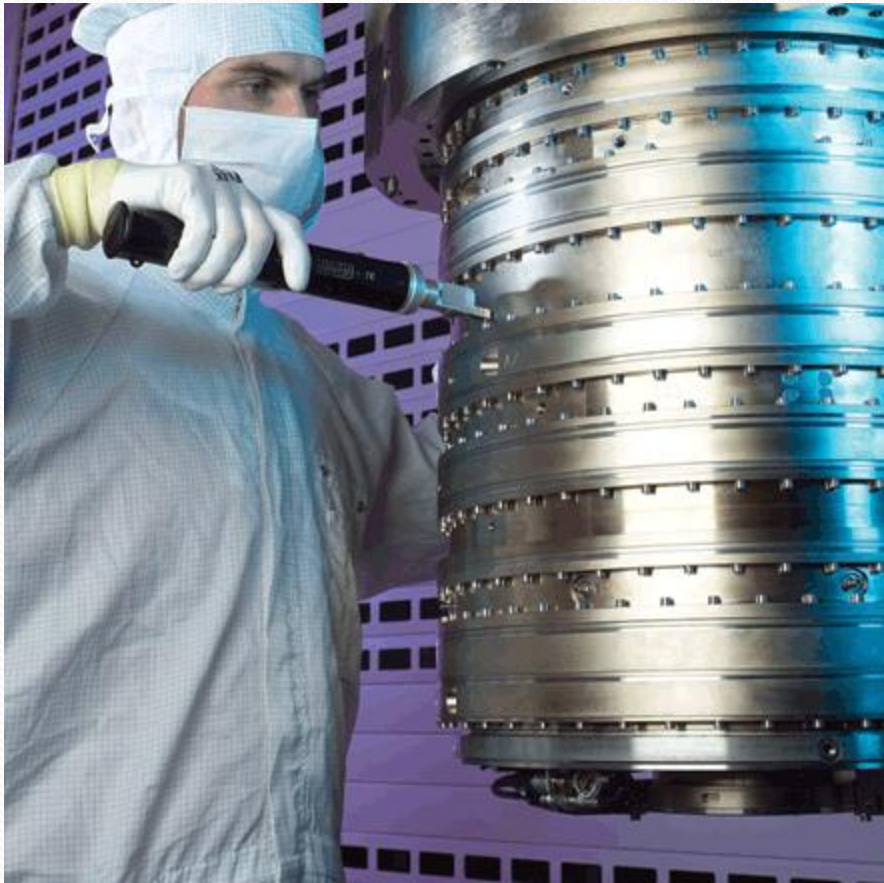
Figure 2 The lens for DUV photolithography with the highest NA: Stariith 1900 from Carl Zeiss. The height of the lens is more than 1 m. The optical design and ray path are schematics and given only as an illustration. The inset depicts a resist structure of 36.5-nm half-pitch, obtained with the lens at full scanning speed. Main image courtesy of Zeiss; inset courtesy of ASML.
