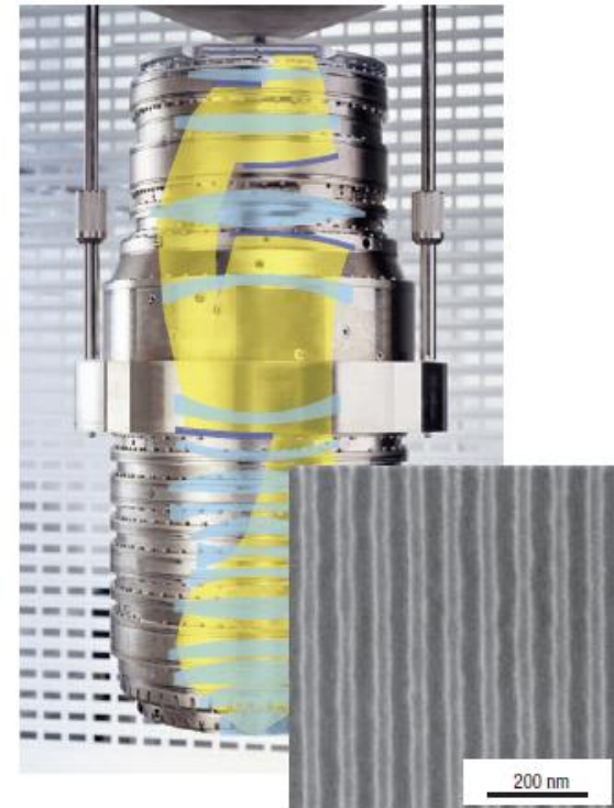
Figure 2 The lens for DUV photolithography with the highest NA: Stariith 1900 from Carl Zeiss. The height of the lens is more than 1 m. The optical design and ray path are schematics and given only as an illustration. The inset depicts a resist structure of 36.5-nm half-pitch, obtained with the lens at full scanning speed. Main image courtesy of Zeiss; inset courtesy of ASML.
