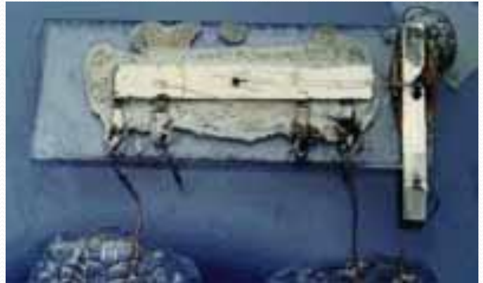
A technological milestone: Kilby's integrated circuit, TI (1959)
