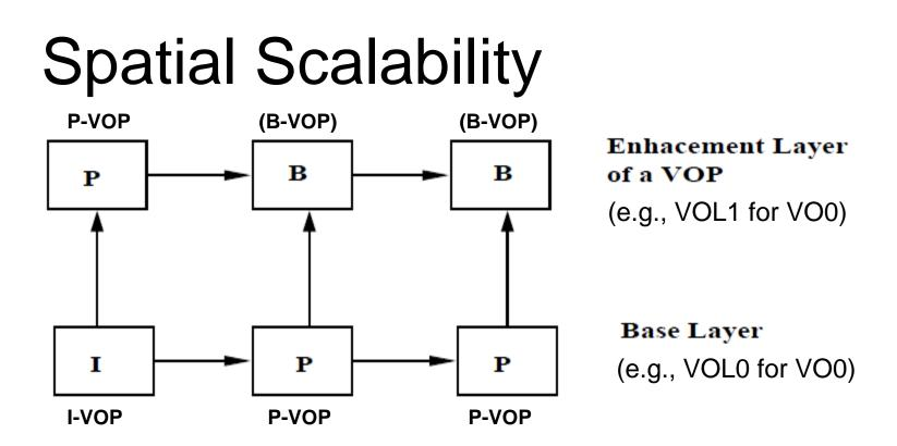
VOP which is temporally coincident with **I-VOP** in the base layer, is encoded as **P-VOP in the enhancement layer**.
