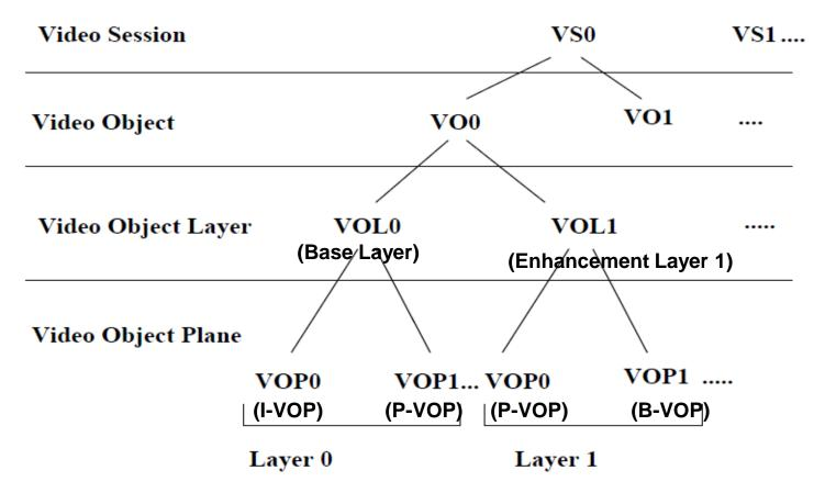
New MPEG-4 Aspect: Object-based layered syntactic structure
