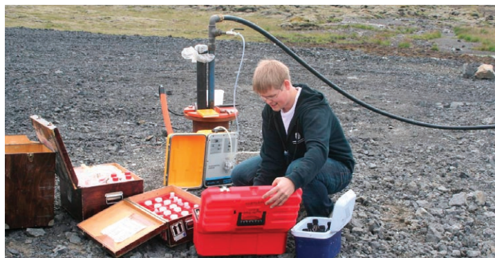
Helgi Arnar Alfreðsson, one of several PhD students in the CarbFix project, sampling one of the monitoring wells at the Hellisheidi site. PHOTO: E. S. EIRKSDÓTTIR
