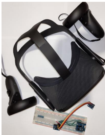
Fig. 5. View of the designed system for determining the position of the human body in the virtual world.
