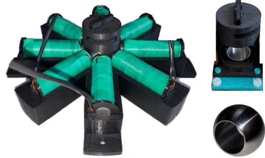
Fig. 11. Current test prototype together with valve body and ball itself
