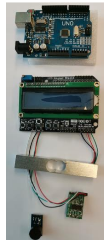
Fig. 2. Electronic components of the scale (from the top: Arduino UNO board, LCD Keypad Shield, tensometric beam with signal conditioning and buzzer at the left lower corner).
