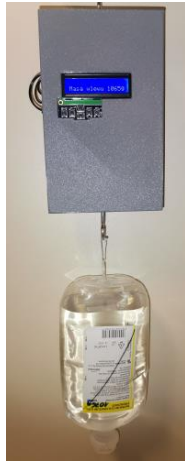
Fig. 4. The developed concept of the infusion fluid level monitoring system.
