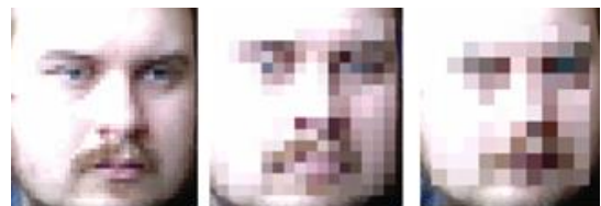
Fig. 7. Censoring the detected face with three different settings
