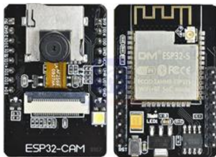
Fig. 2. ESP32-CAM IoT Device
