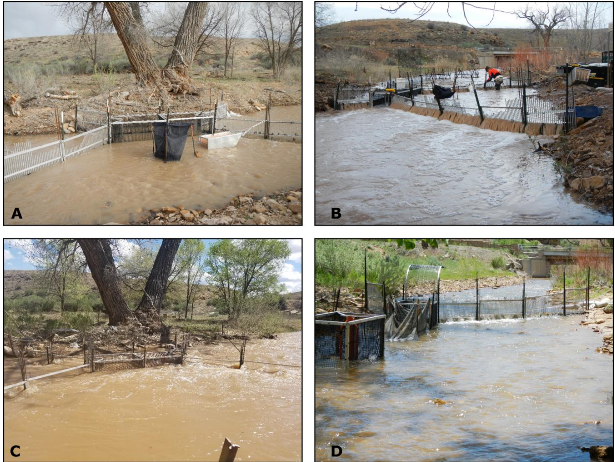
Figure 2.3. The Cottonwood Creek fish weir under a variety of conditions. Panel A shows the fully operational weir in 2016 when flows were low but ascending. In panel B, the 2016 weir is shown fully functional, but at flows approaching damaging levels. Leaf matter and woody debris had to be cleaned nearly continuously at these levels. High flows forced the removal of pickets or fence sections in both years (panel C; 2017 pictured here) to preserve the integrity of the overall structure. Fish had free access to the creek under these conditions. In 2016 especially, the outmigration occurred in such mass that fish threatened the integrity of the weir as can be seen in panel D - the damming effect seen on the upper fence is the result of several hundred fish attempting to pass the weir simultaneously.
