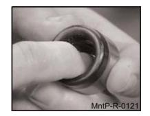
2. Insert cup and cross. Drive in with spacer.
