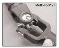
8. Grease Kit after assembly is completed.
