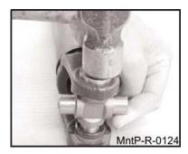
**5.** Drive cup down with spacer and insert snap ring
