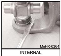
Position joint in loose vice, strike top arm of unsupported yoke to drive the top cup up. Repeat on opposite side.
