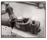
3. If you cannot grip the loosened cap per Step 4, use a pointed tool to tip a needle them repeat Step 2.
