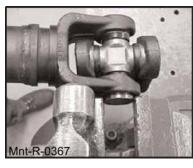
Support cross in loose vise and strike yoke arm. Repeat Step 4 to remove remaining two cups.
