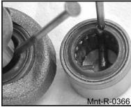
**4.** Grip loosened cup in vise, strike yoke arm to drive yoke off cup. Repeat on opposite cup.
