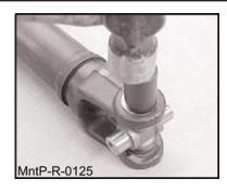
**6.** To loosen cross, strike yoke arm and check cross for free rotation
