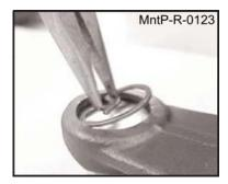
**4.** Insert second cup and hold cross into cup. Drive cup flush with arm.
