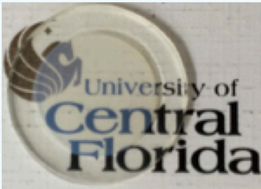
The UCF logo displayed through a transparent CaF 2 -acrylate nanocomposites containing over 84 wt% CaF 2 .
