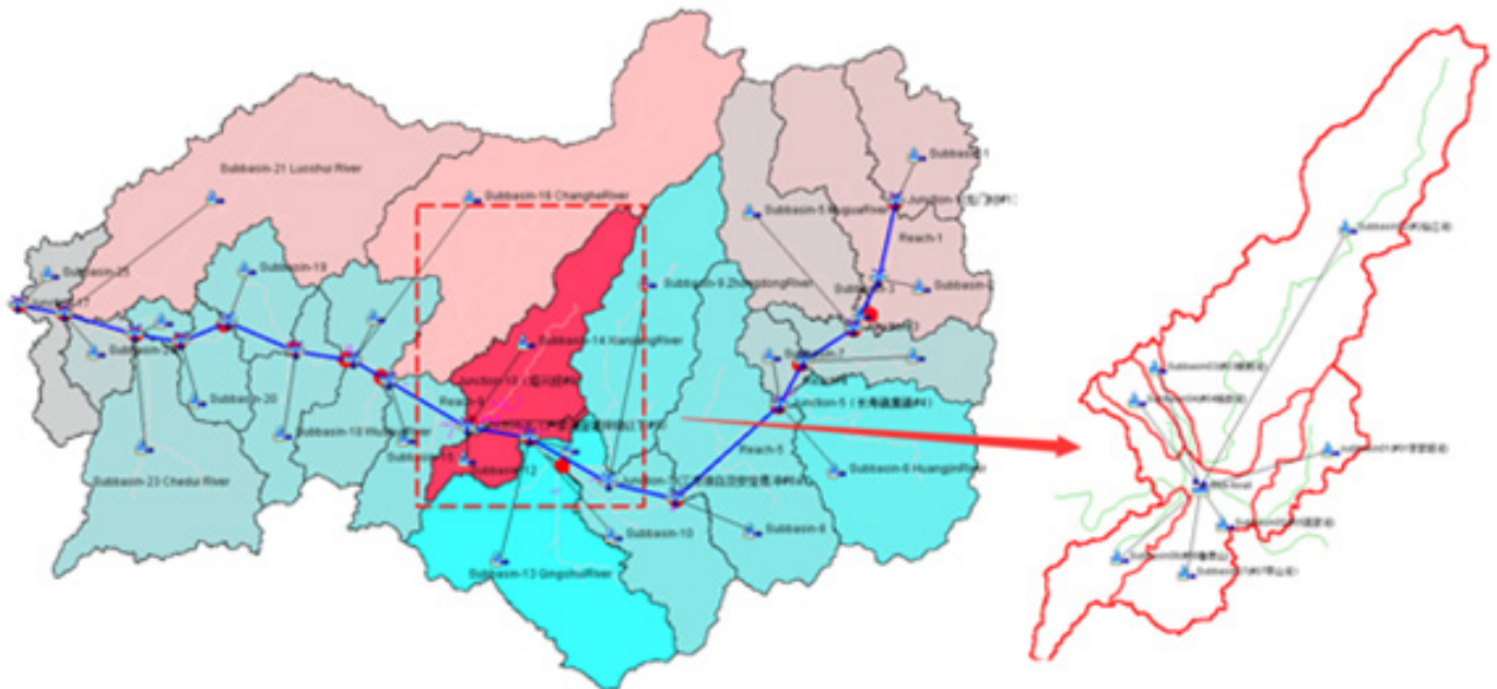
Figure 5: Distributed hydrologic model for rainfall-runoff modeling. (a) Basin model for rural area. (b) Basin model for urban area.
