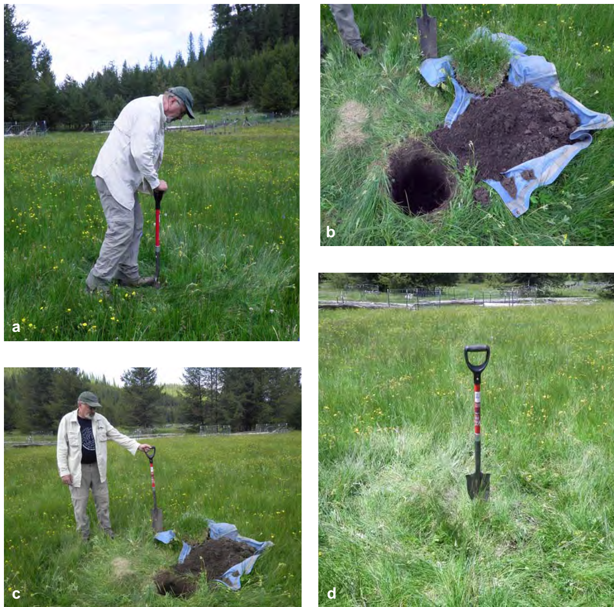
Figure 4. A series of 4 images depicting soil pit excavation and rehab of pit after completion of soil description, including (from upper left), (a) excavation using tile spade, (b) completed soil pit with intact organic surface plug and excavated soil on tarp, (c) close up of completed soil pit, and (d) soil pit filled in with surface plug in place and rehabilitation complete. Riparian vegetation mapping study in the Grande Ronde River watershed, Oregon, 2014.
