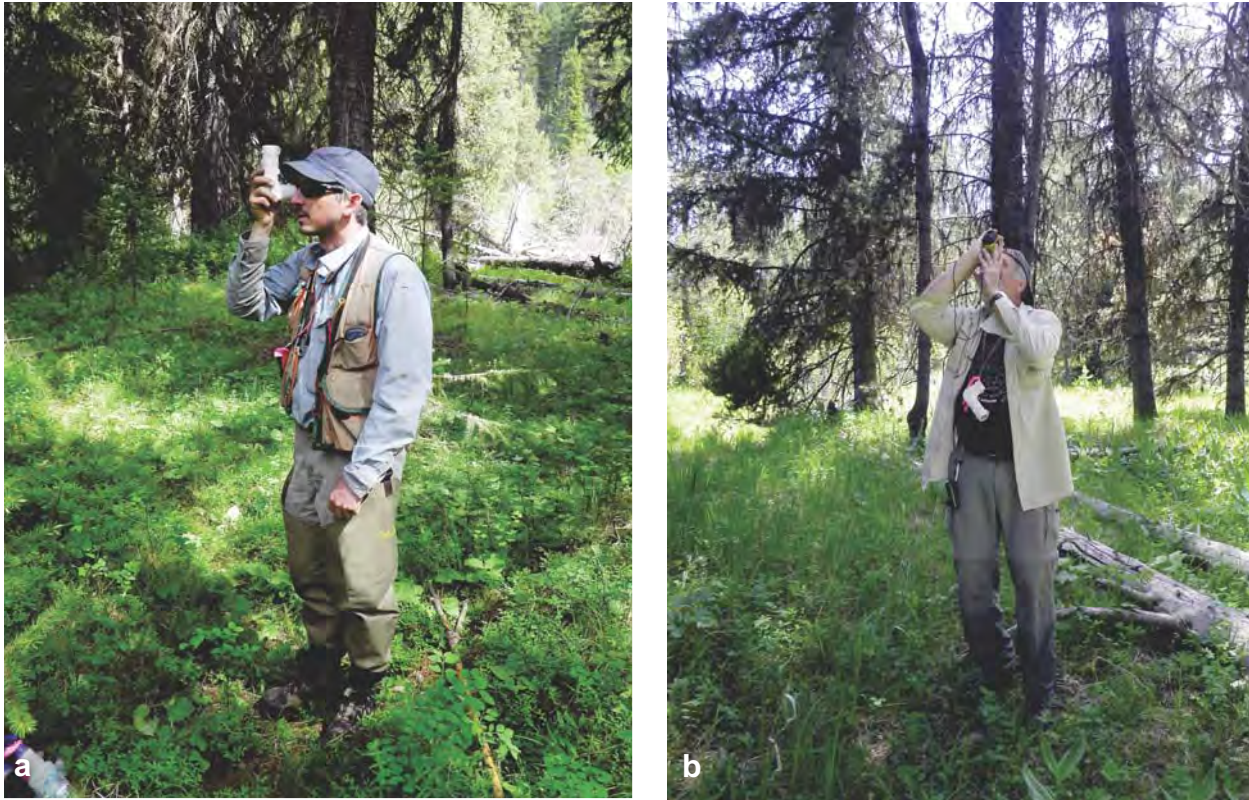
Figure 6. Photographs illustrating data collection at LiDAR plots, including use of a densitometer to estimate canopy density (a), and use of a laser rangefinder to estimate tree and tall shrub heights (b). Riparian vegetation mapping study in the Grande Ronde River watershed, Oregon, 2014.
