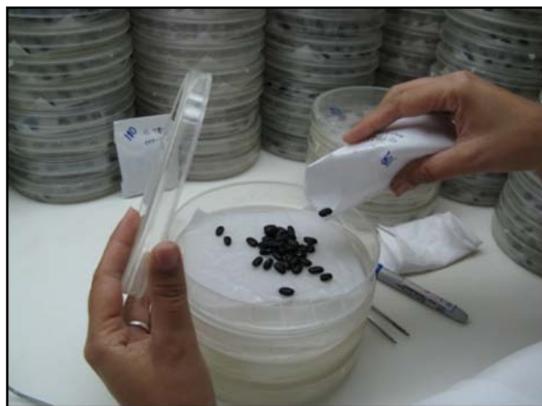
Figure 7. Bean seeds being deposited in petri dishes with paper moistened with distilled water (Blotter technical test).
