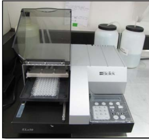
Figure 42. Automatic microplate washer (Every cycle of washing in this machine lasts approximately 6 minutes).
